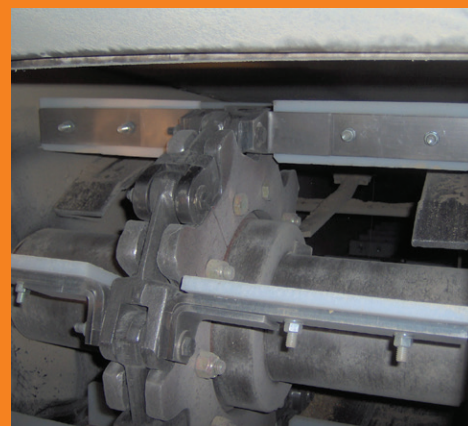
UHMW Paddles on "T" Plate Flights – Drive End
