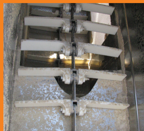
Feed Mill Application using Bolt 'N' Go Chain with Nylon Flights
