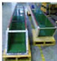
Chute and vibration chute
